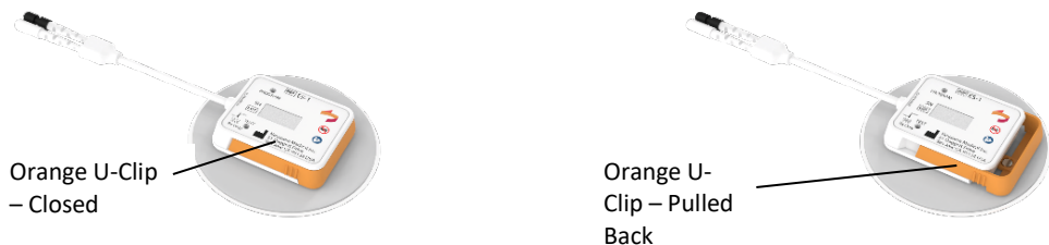
Figure 3. External Stimulator with Orange U-Clip. Closed (Left); Pulled Back (Right)
