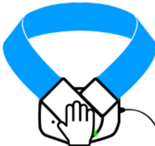
Figure 14 – Tapping on the Charger while it is on the Docking Station will show its battery level.
