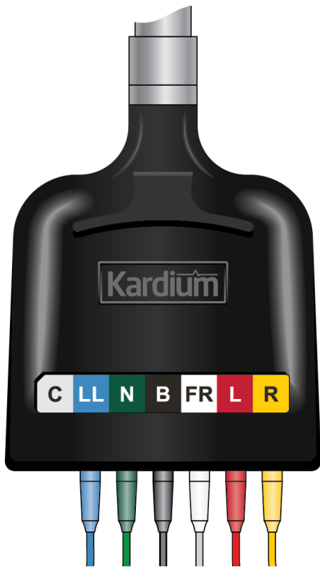
Figure 83: GPS Electrodes connected to the GPS Cable
