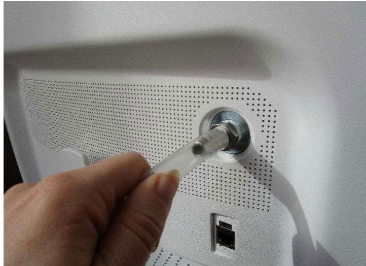
Figure 15: Connect vacuum tubing to the Claire OCT System vacuum port
