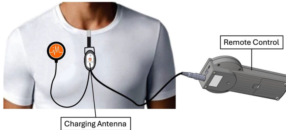
Figure 3. Patient IPG Charging Configuration
