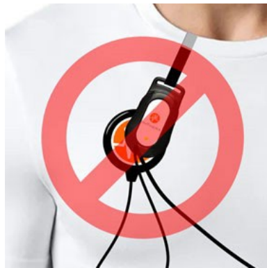
Figure 8. Unsafe Charging Configuration
