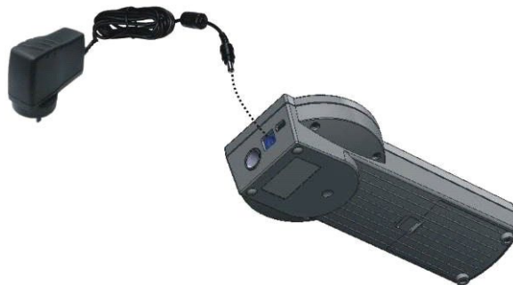
Figure 6. Connect Power Cord to RCC
