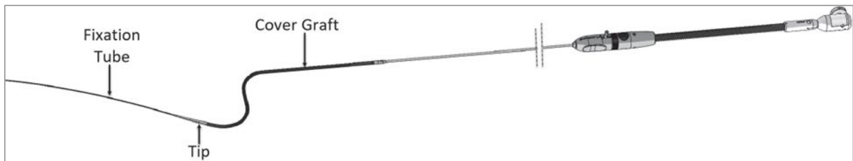
Figure 6. NEXUS® Arch Stent Graft Delivery System – Pre-Shaped (thunderbolt shape)
