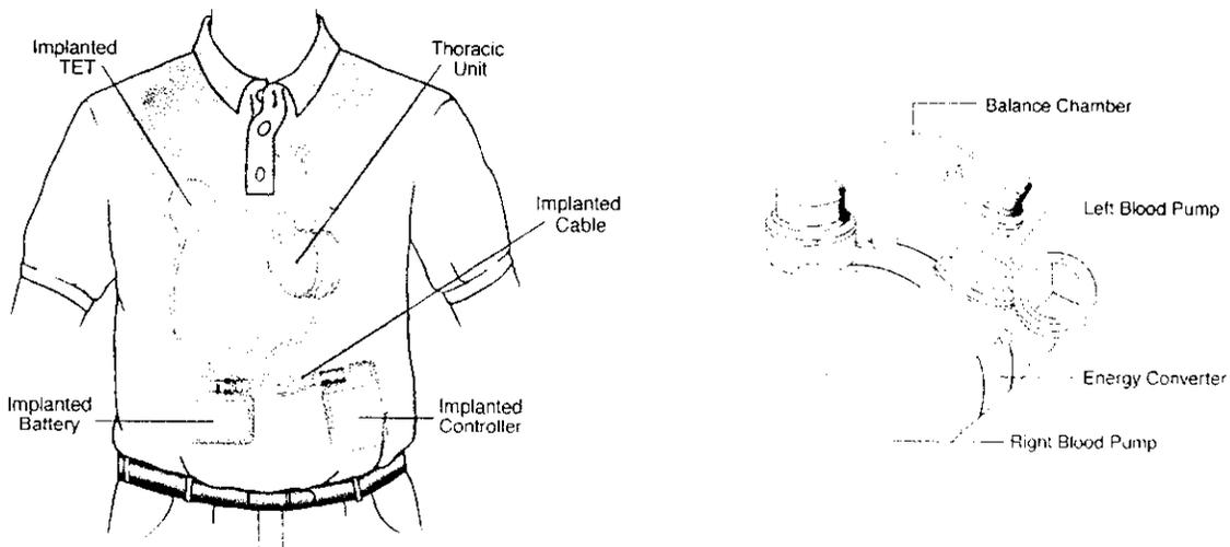
Figure 1. Implanted components
