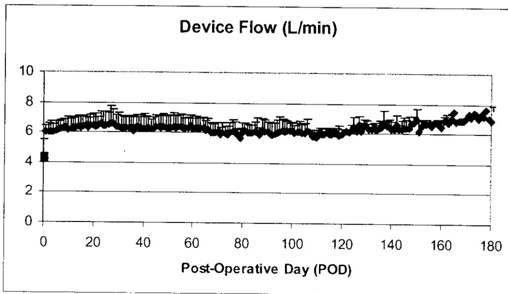
Figure 6. Pump Output
