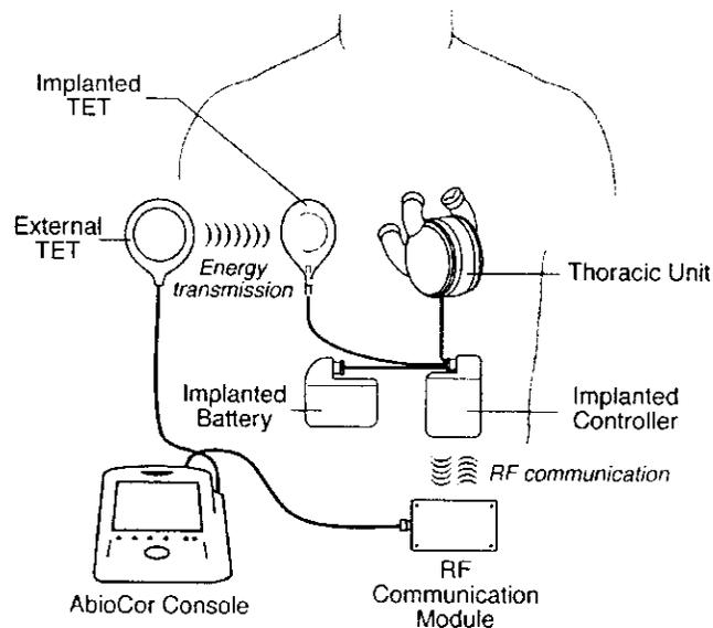
Figure 2. External components and their functional relationship with the implanted parts
