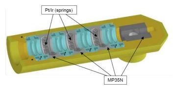
The DF4 module is integrated into the header of the Ilesto/Iforia DF4 variants. In addition to the DF4 module, the entrance bore of the header is modified to be compatible with the module and to comply with the ISO standard. Pin and spring contacts are connected using connection bands with the same ICD/CRT-D feed throughs and materials as in the DF-1 variants.
