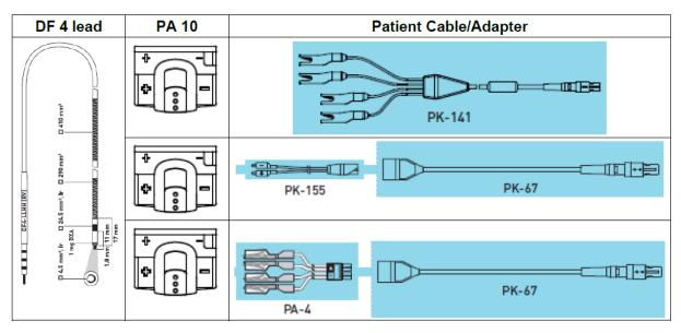
PA 10 is used for transmission of sensing signals and pacing pulses for diagnostics and therapy during the implant procedure (i.e. connection to the pacing system analyzer). The PA 10 adapter does not contact the DF4 ring contacts of the shock coil conductors. The PA 10 is only provided as a separately available sterile accessory.
