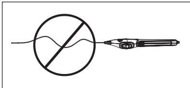
**Caution:** Any slack in the stent system (outside the patient) could result in deploying the stent beyond the target site.
