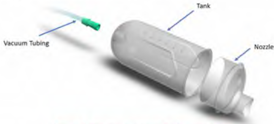
Figure 1: Schematic image of the Bateman Bottle.
