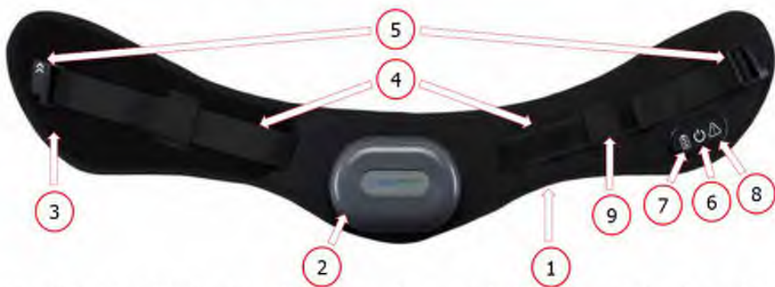
Figure 1. Front view of the Osteoboost: (1) Nylon-covered neoprene belt, (2) vibration pack (housed on the back of the neoprene belt), (3) inner Velcro, (4) nylon straps, (5) clasp, (6) power button, (7) battery status light, (8) attention light, (9) hip accelerometer (located in the neoprene belt).
