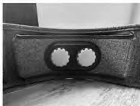
Figure 1. Inner Surface of Sonu Headband Showing Medical-Grade Silicone Transducer Covers
