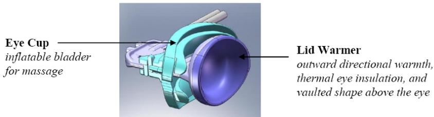
In this cross-sectional representation, the Disposable positions around the eyelids during device use:
