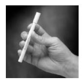
(2) Crush the bottom ampule containing the solution vehicle by applying finger pressure to Position A on the cardboard sleeve.
