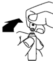
To break, place thumb on the dot and snap back.
