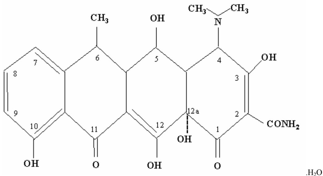
with an empirical formula of C<sub>22</sub>H<sub>24</sub>N<sub>2</sub>O<sub>8</sub>·H<sub>2</sub>O and a molecular weight of 462.46. The chemical designation for doxycycline is 2-Naphthacenecarboxamide, 4-(dimethylamino)-
