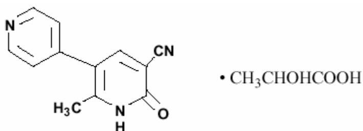
Milrinone is an off-white to tan crystalline compound with a molecular weight of 211.2 and an empirical formula of C<sub>12</sub> H<sub>9</sub> N<sub>3</sub> O. It is slightly soluble in methanol, and very slightly soluble in chloroform and in water. As the lactate salt, it is stable and colorless to pale yellow in solution. PRIMACOR is available as sterile aqueous solutions of the lactate salt of milrinone for injection or infusion intravenously.
