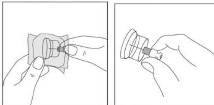
3. Place vial on a hard surface. Hold the base of the vial. Orient the SmartSite® Access Device vertically over the vial so that the spike tip is at the center of the vial's rubber stopper. With a straight downward push, press the spike tip of the SmartSite® Access Device through the center of the vial's rubber stopper until the device securely snaps onto the vial top.
