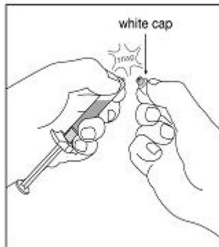
For all syringe assembly steps, hold the syringe only by the white collar located at the tip of the syringe. Be careful to not overtighten components when assembling. Overtightening connections may cause syringe component parts to loosen from the syringe body.
