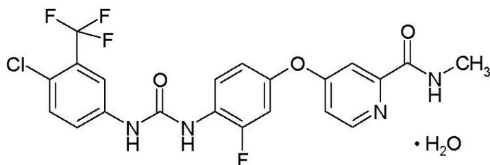
Regorafenib is a monohydrate and it has a molecular formula  $C_{21}H_{15}ClF_4N_4O_3 \cdot H_2O$  and a molecular weight of 500.83. Regorafenib is practically insoluble in water, slightly soluble in acetonitrile, methanol, ethanol, and ethyl acetate and sparingly soluble in acetone.
