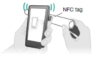
1) Hold the NFC tag against the back of the smartphone, making sure the label contacts the smartphone's back.
