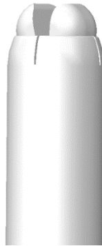
Figure 6: Close-up of Hemispherical Dome at Tip of Tube
