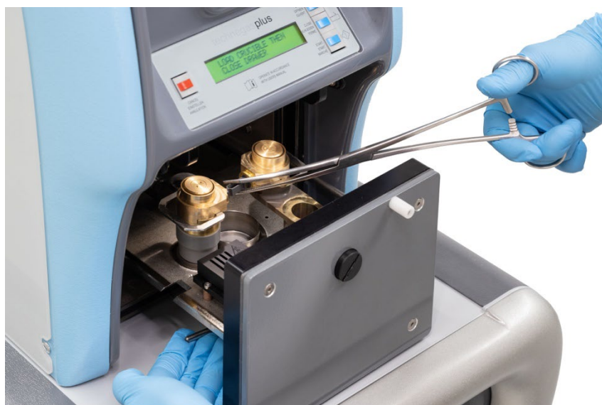
Figure 11: Installing the Technegas Crucible into the TP Drawer
