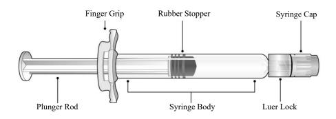
**Step 1:** Holding the Luer lock in one hand (avoid holding the plunger rod or syringe body), unscrew the syringe cap by twisting it counter-clockwise with the other hand.
