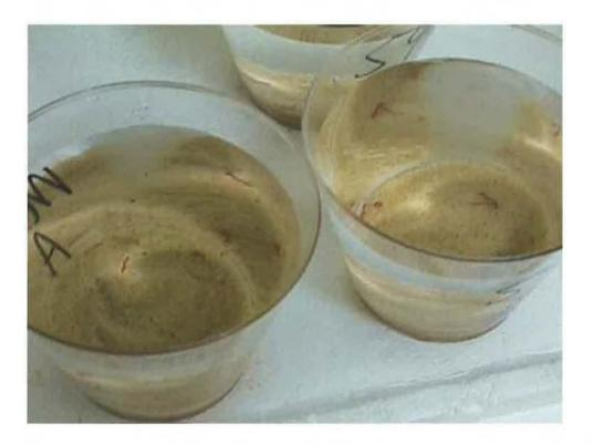
A6-6. Close-up of chironomid test chambers with sterile sand on cup bottoms.
