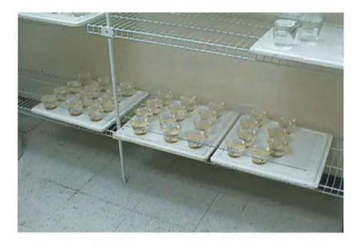
A6-4. Chironomid acute toxicity test setup. Temperature and light controlled room.
