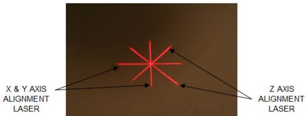
Figure 3-14. Red Crosshairs X & Y Axes, Red Crosshairs Z Axis Alignment
