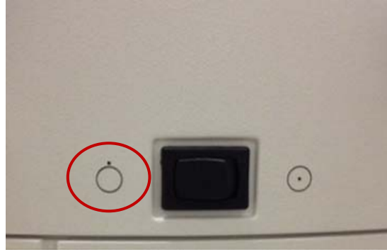
Figure 3-23. Power Off Position
