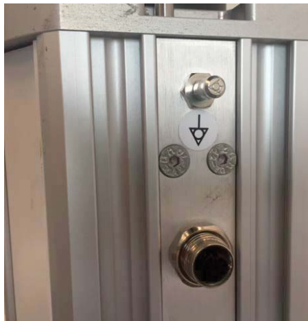
Figure 24: Potential compensator conductor
