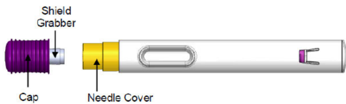
Figure 1.c Illustration of Vedolizumab SC PFS+AI Device Constituent Cross-section View of AI after Cap Removal
