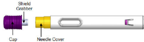
Figure 1.b Illustration of Vedolizumab SC PFS+AI after Cap Removal
